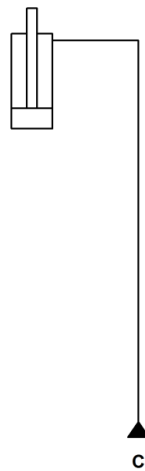
Hydraulic flow chart three-point linkage 8 Single cylinder
